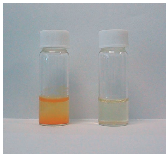
Figure 1. Photograph of 6T (left) and a mixture of 6T and CMA (right) in 10% aqueous DMSO at pH 10.5.
